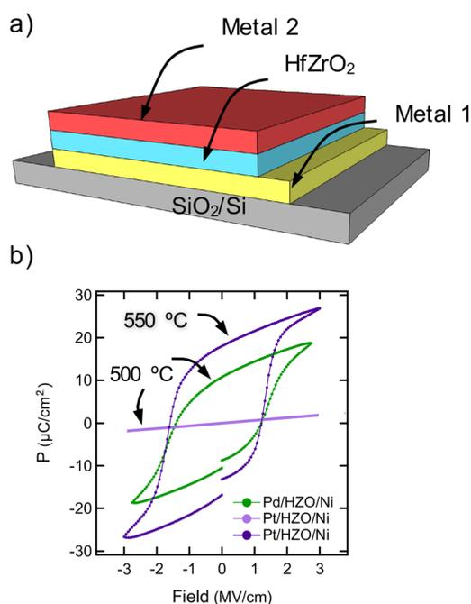
FIG. 1. (Color online) MFM structure and the impact of annealing temperature on ferroelectric behavior. (a) Schematic of parallel-plate MFM capacitors with the structure of metal 1/HZO/metal 2. Metals 1 and 2 refer to the bottom and top electrodes, respectively. (b) P-E curves of Pt/20 nm HZO/Ni and Pd/20 nm HZO/Ni demonstrating how the temperature for driving ferroelectric behavior depends on the capping layer stack.
