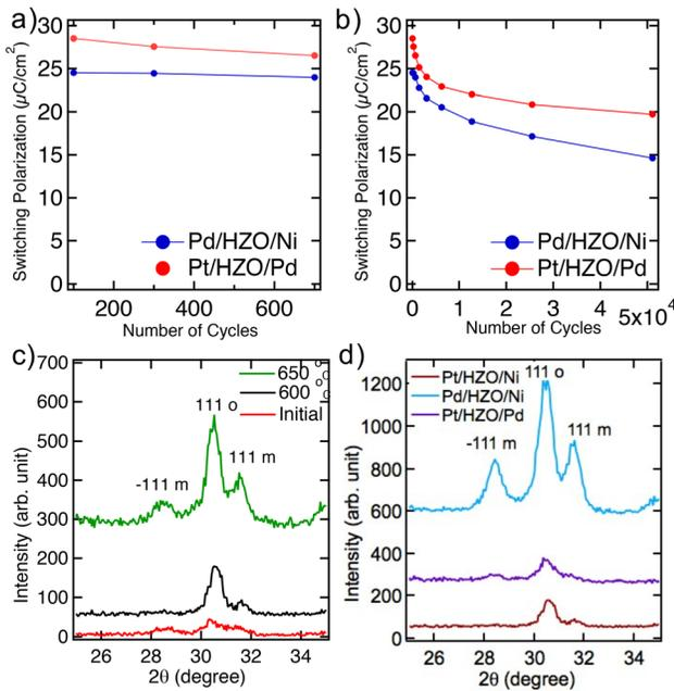
Fig. 4. (Color online) (a) Retention and (b) fatigue testing at 1 kHz with an applied voltage of 4 V for Pd/20 nm HZO/Ni and Pt/20 nm HZO/Pd MFM capacitors annealed at 700 °C. (c) GAXRD for Pt/20 nm HZO/Ni initially and after different annealing temperatures. (d) GAXRD for Pt/20 nm HZO/Ni, Pd/20 nm HZO/Ni, and Pt/20 nm HZO/Pd MFM capacitors.
