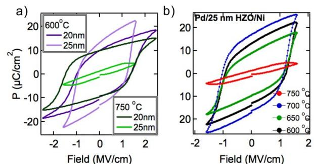
Fig. 3. (Color online) Postanneal P-E curves at various annealing temperatures from MFM capacitors comprised of Pd/HZO/Ni with varying HZO thicknesses of (a) 20 and 25 nm and (b) 25 nm.
