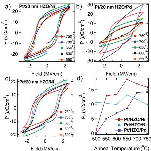
Fig. 2. (Color online) P-E curves from MFM capacitors with different metal capping layer stacks, annealed at various temperatures. The MFM stacks are (a) Pt/20 nm HZO/Ni, (b) Pt/20 nm HZO/Pd, and (c) Pd/20 nm HZO/Ni. (d) Average  $P_r$  vs annealing temperature from Pt/HZO/Ni, Pt/HZO/Pd, and Pd/HZO/Ni with a HZO thickness of 20 nm.
