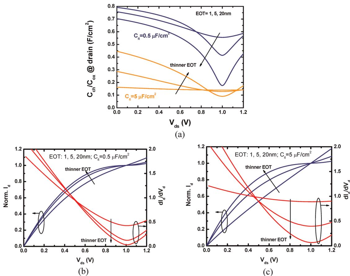
Figure 3. (a) Calculated  $C_{ch}/C_{ox}$  as a function of drain-source voltage at the drain-end for devices with nonzero interface traps. (b) Simulated output characteristics for 500 nm channel device with EOT = 1, 5, 20 nm and  $C_{it} = 0.5 \mu F/cm^2$ . (c) Simulated output characteristics with  $C_{it} = 5 \mu F/cm^2$ .
