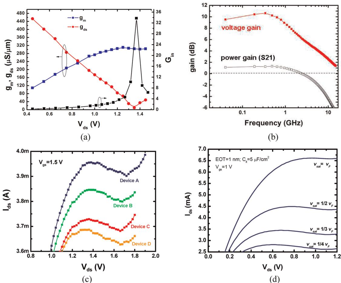
Figure 4. (a) Measured  $g_m$ ,  $g_{ds}$ , and  $G_m = g_m/g_{ds}$  across a range of drain bias at  $V_{gs} = 1.2$  V. (b) Measured frequency response of extrinsic voltage gain and power gain (S21) from s-parameter measurements. (c) Measured NDR effect from four devices on the same chip. (d) Simulated  $I_{ds}$ – $V_{ds}$  with various  $v_{sat}$ .
