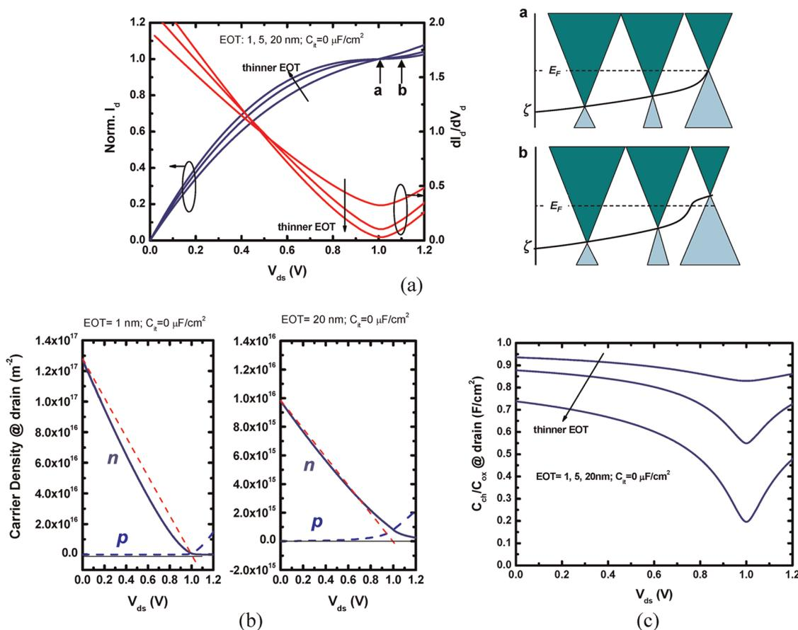
Figure 2. (a) Simulated output characteristics for 500 nm channel device with EOT = 1, 5, 20 nm.  $C_{it} = 0 \mu\text{F}/\text{cm}^2$  is assumed. (b) Simulated electron density and hole density at the drain-end for devices with EOT = 1 nm (left) and 20 nm (right). (c) Gate to channel capacitance normalized to  $C_{ox}$  as a function of drain–source voltage at the drain-end.
