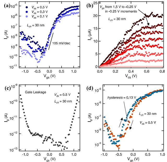
**Figure 4.** Characteristics of fully self-aligned GAA-CNTFET having a single nanotube channel with  $L_{gate} \approx 30$  nm. (a) Subthreshold curves showing good switching behavior. (b) Output curves exhibiting saturation at  $\sim 0.45$  V and high on-current ( $\sim 20$   $\mu$ A at  $V_{gs} - V_{th} = 1.25$  V). (c) Gate leakage indicating stable operation up to  $\sim 1.3$  V. (d) Double sweep subthreshold curves showing small hysteresis in the device.
