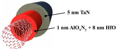
**Figure 3.** Illustration of the gate-all-around stack consisting of an annularly coated high-k dielectric and conductive TaN gate metal.
