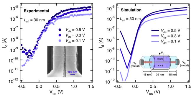
**Figure 7.** Comparison of experimental characteristics with NEGF simulation that approximates the device structure, including a fixed charge density  $N_d = 0.4/\text{nm}$ .
