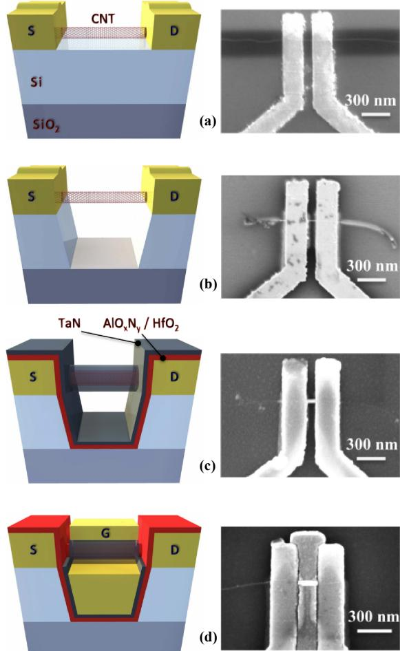
**Figure 1.** Process flow for fabricating self-aligned, gate-all-around CNTFETs; each step is illustrated with a cross-sectional schematic and corresponding top-view SEM image. (a) CNTs placed on SOI substrate and Pd source/drain contacts formed. (b) Anisotropic wet etch of Si in KOH causing CNT channel to be suspended. (c) Gate dielectric and metal deposited on CNT channel using ALD. (d) Self-aligned gate contact formed and TaN cleared from field.
