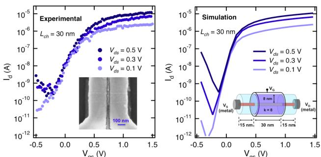
**Figure 7.** Comparison of experimental characteristics with NEGF simulation that approximates the device structure, including a fixed charge density  $N_d = 0.4/\text{nm}^2$ .
