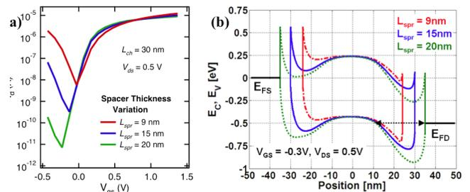
**Figure 8.** Simulation results showing the impact of the spacer thickness on the operation of a GAA-CNTFET with  $N_d = 0.4/\text{nm}$ . (a) Subthreshold curves showing a decrease in *off*-state leakage as the spacer thickness is increased. (b) Corresponding band diagrams illustrating the thinning of the tunnel barrier at the drain-end that causes more ambipolar leakage in thinner spacer devices.
