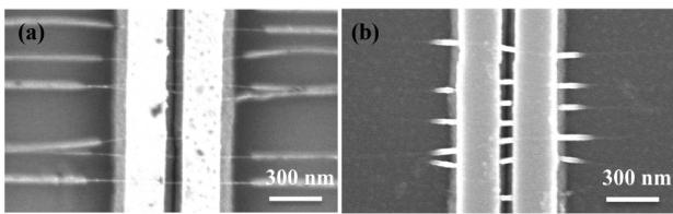
**Figure 2.** Top-view SEM images (a) after Si etch and (b) after ALD of gate-all-around dielectric and metal. Note how the CNTs are suspended between the metal contact lines in (a) and touch the substrate further away from the contacts. Likewise, only the suspended portion of the CNTs are annularly coated and thus visible in (b).
