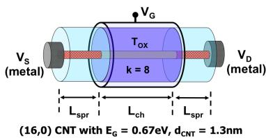
**Figure 6.** Schematic of GAA-CNTFET structure used in NEGF simulations. The spacers ( $L_{spr}$ ) are the same dielectric and thickness as the gate dielectric in the experimental devices. A fixed charge density ( $N_d$ ) is applied across the channel to represent the fixed charge from the ALD dielectric.
