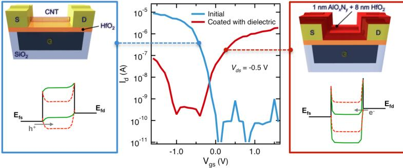
an n-FET (see Fig. 5). All GAA-CNTFETs with this dielectric stack operate as n-FETs despite the use of high work function Pd contacts. This polarity shift is attributed to positive fixed charges in the HfO<sub>2</sub>.
