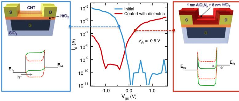
**Figure 5.** Subthreshold curves from same bottom-gated CNTFET before/after coating with dielectric stack that was used for the GAA devices. As illustrated in the band diagrams (green bands and red bands depict *on*-state and *off*-state, respectively), the GAA dielectric contains strong positive fixed charge that acts as doping across the CNT channel, converting the device from a p-FET to an n-FET.
