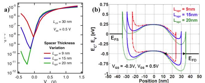
**Figure 8.** Simulation results showing the impact of the spacer thickness on the operation of a GAA-CNTFET with  $N_d = 0.4/\text{nm}^2$ . (a) Subthreshold curves showing a decrease in *off*-state leakage as the spacer thickness is increased. (b) Corresponding band diagrams illustrating the thinning of the tunnel barrier at the drain-end that causes more ambipolar leakage in thinner spacer devices.
