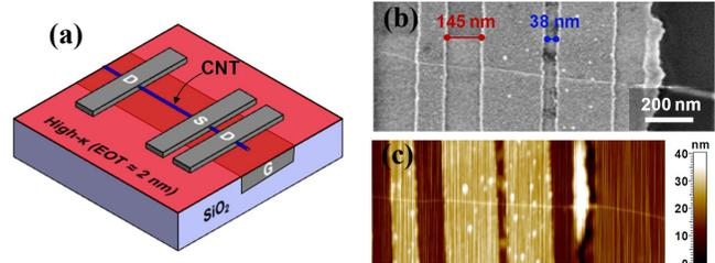
**Figure 1.** (a) Schematic, (b) scanning electron microscope (SEM), and (c) atomic force microscope (AFM) images showing a semiconducting CNT on top of an LBG (Pd), with Pd electrodes forming two different channel length devices. The dielectric is 10 nm  $\text{HfO}_2$  with  $\kappa \approx 18$ , yielding an  $\text{EOT} \approx 2$  nm. AFM was used to determine the CNT diameter,  $d_{CNT} \approx 1.2$  nm.
