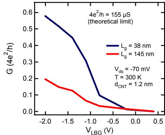
**Figure 4.** Conductance at room temperature for two different channel length devices on the same CNT, illustrating the clear advantage that scaling has for the on-state. The 38 nm device exhibits the highest conductance ever reported for a semiconducting CNT that has a demonstrated  $I_{on}/I_{off} > 10^2$  (present device has  $I_{on}/I_{off} > 10^5$ ).
