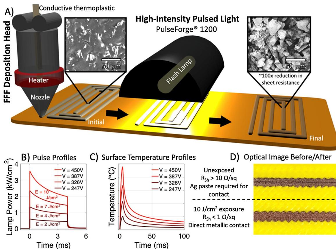
Fig. 1. Schematic diagram of the FFF printing and pulsed-light exposure process. A) Illustration of the FFF printing and pulsed light exposure process with filament surface morphology highlighted before and after exposure. B) Calculated power profiles emitted from the flash lamp at various capacitor bank voltages. C) Qualitative plot of simulated surface temperature values on ABS during and after exposure. D) Optical comparison of as-printed versus exposed filament.
