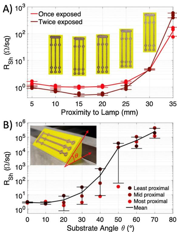
Fig. 4. Exposure effects associated with part orientation. A) Plot of sheet resistance versus part proximity from lamp window with optical images provided in the insets indicating color changes as part is moved away from lamp at a constant exposure condition (V = 450 V, PW = 4 ms). B) Plot of sheet resistance versus part angle with colored data points indicating which 4-point probe structures were closest to or furthest from the lamp during exposure (V = 450 V, PW = 4 ms).
