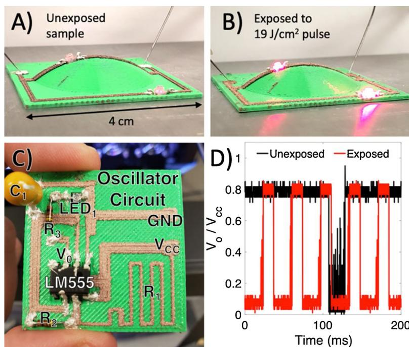
Fig. 5. Pulsed-light exposed 3D printed circuit boards. A-B) Images of non-planar LED circuits driven at 2 V a) without and b) with pulsed-light exposure. C) Image of a 3D printed oscillator circuit board and interconnects with placed-in components adhered with silver epoxy. D) Output signal ( $V_o/V_{cc}$ ) waveform of oscillator circuits prepared with and without pulsed-light exposure.
