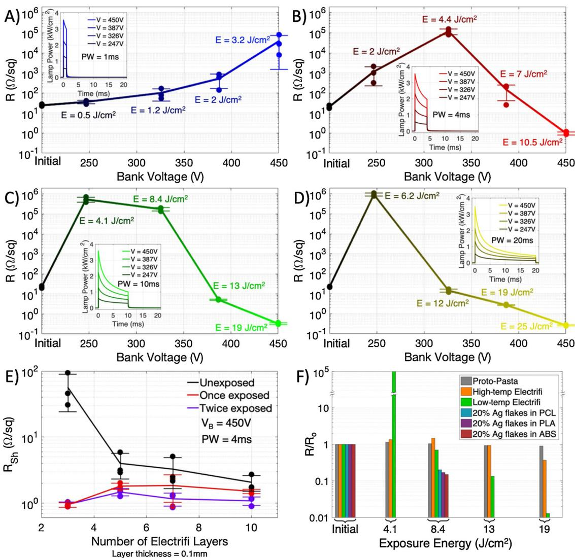
**Fig. 3.** Electrical characterization of pulsed-light exposed 3D printed filament. A-D) Sheet resistance of 3D-printed Electrifi with varying exposure conditions (bank voltage, pulse width) with pulse profiles provided in the insets. E) Sheet resistance plotted with an increasing number of printed Electrifi layers for unexposed, once-exposed and twice-exposed films. F) Sheet resistance comparison across various conductive filaments and exposure conditions.
