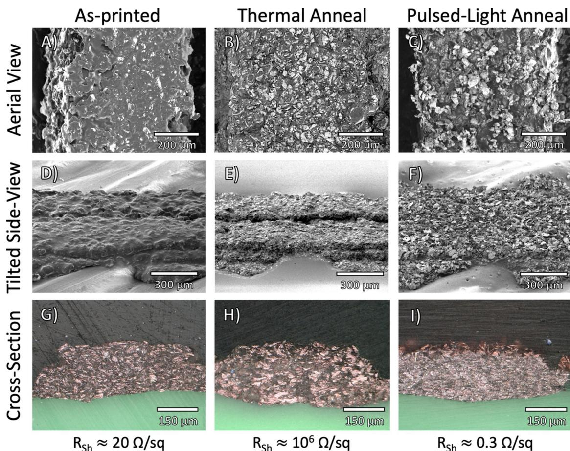
Fig. 2. SEM and optical analysis of conductive composite filament. A-C) SEM images of the surface of as-printed, thermally annealed, and pulsed-light annealed copper-loaded filament from an aerial view. D-F) SEM images of as-printed, thermally annealed, and pulsed-light annealed copper-loaded filament from a side view. G-I) Cross-sectional optical images of as-printed, thermally annealed, and pulsed-light annealed copper loaded filament cast in polished epoxy.
