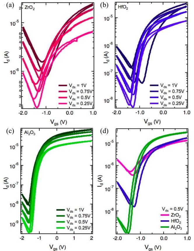
**FIGURE 2. Impact of dielectric type on 2D NC-FET performance. Subthreshold curves with small, counterclockwise hysteresis for devices with 4 nm HZO and 4 nm (a) ZrO<sub>2</sub>, (b) HfO<sub>2</sub>, and (c) Al<sub>2</sub>O<sub>3</sub> as the gate oxide at multiple drain biases. (d) Comparative curves for devices at  $V_{ds} = 0.5$  V. All devices have  $L_{ch} = 500$  nm.**
