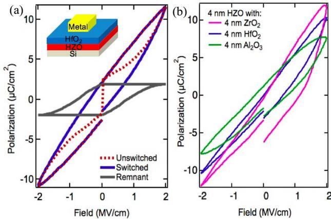
**FIGURE 3.** Polarization - electric field (P-E) curves for the various gate stacks studied after a 550 °C RTA for 30 secs. The metal used to contact the stacks for collecting the data is 5 nm Ti/20nm Au. (a) Measured polarization of 5 nm HfO<sub>2</sub>/12nm HZO excluding the impact of leakage current and (b) polarizations of each 4 nm dielectric with 4 nm HZO. Ferroelectric behavior is demonstrated by the nonlinear polarizations.
