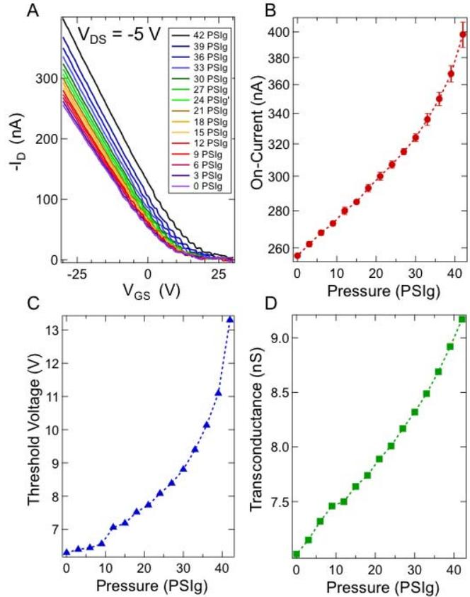
Fig. 3. Modulation of electrical parameters of the CNT-TFT corresponding with environmental pressure change. (A) Characteristic transfer curves for each PSIG measured at a drain to source voltage ( $V_{DS}$ ) of  $-5$  V. (B) On-current, (C) threshold voltage, and (D) transconductance with respect to the environmental pressure.
