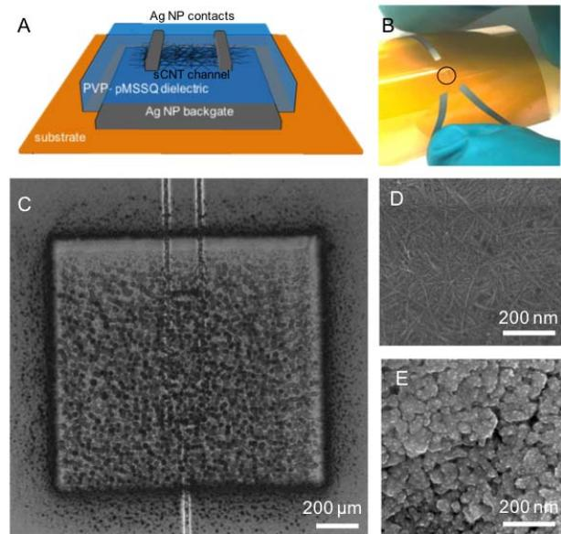
Fig. 1. Fully printed CNT-TFT structure and morphology. (A) Schematic of the fully printed, bottom-gate, top-contact CNT-TFT. (B) Photograph of the sensor on a Kapton substrate being flexed, with the active device area circled. (C) Optical image at 2.5x zoom of the complete device. SEM images of (D) the CNT thin-film channel and (E) the printed Ag NP source, drain, and back gate.
