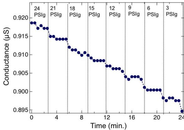
Fig. 5. Conductance changes over time of a printed CNT-TFT pressure sensor. The pressure of the chamber in which the sensor sits is overlaid and ranges from 24 PSiG to 0 PSiG. All values were measured using a voltage divider circuit and an Arduino microcontroller, the values were communicated outside of the chamber using a Bluetooth module.
