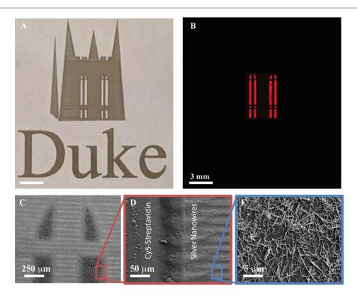
**Figure 5.** Mixed-material ultrasonic aerosol jet printing. (A) Optical photograph of the Duke Chapel and 'Duke' printed with silver nanowires, and the windows printed with Cy5-streptavidin. (B) Fluorescence image (measured at 647 nm) of same print area showing the localized regions of printed biological ink. SEM images of (C) the window region of the print and higher magnification views of (D) the interface between the silver nanowires and streptavidin and (E) the silver nanowires.
