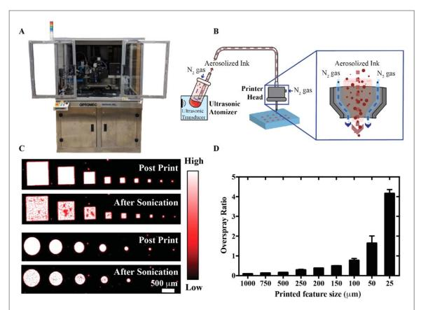
**Figure 1.** Aerosol jet printed biological ink. (A) Optomec Aerosol Jet 300 printer used in this work. (B) Schematic representation of ultrasonic atomization Aerosol Jet Printing (u-AJP), with a magnified view of the printer head. (C) Fluorescence images showing intensities for squares and circles of printed Cy-5 labeled BSA, captured under 647 nm light before (top) and after (bottom) sonication. (D) Overspray ratio of the aerosol jet printed shapes as a function of printed feature size.
