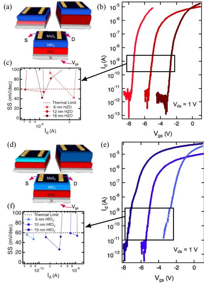
**FIGURE 1. Impact of ferroelectric and dielectric thickness on 2D NC-FETs.**
