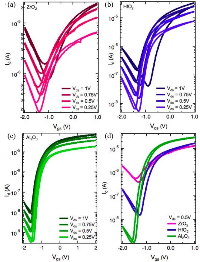
**FIGURE 2. Impact of dielectric type on 2D NC-FET performance.**
