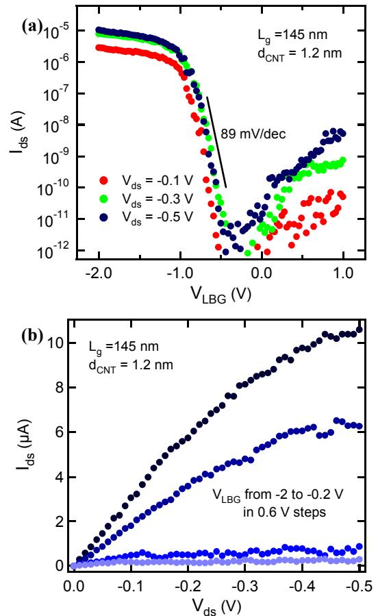
**Figure 3.** Characteristics of  $L_g = 145$  nm channel device from the same CNT as in Fig. 2. (a) Subthreshold plot for different  $V_{ds}$  with  $SS \approx 89$  mV/dec. (b) Output curves for different  $V_{LBG}$  showing the beginning of saturation and current of  $\sim 7$   $\mu$ A at 0.5 V overdrive ( $V_{LBG} - V_{th} = V_{ds} = -0.5$  V).
