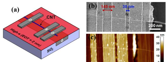
**Figure 1.** (a) Schematic, (b) scanning electron microscope (SEM), and (c) atomic force microscope (AFM) images showing a semiconducting CNT on top of an LBG (Pd), with Pd electrodes forming two different channel length devices. The dielectric is 10 nm  $\text{HfO}_2$  with  $\kappa \approx 18$ , yielding an  $\text{EOT} \approx 2$  nm. AFM was used to determine the CNT diameter,  $d_{CNT} \approx 1.2$  nm.
