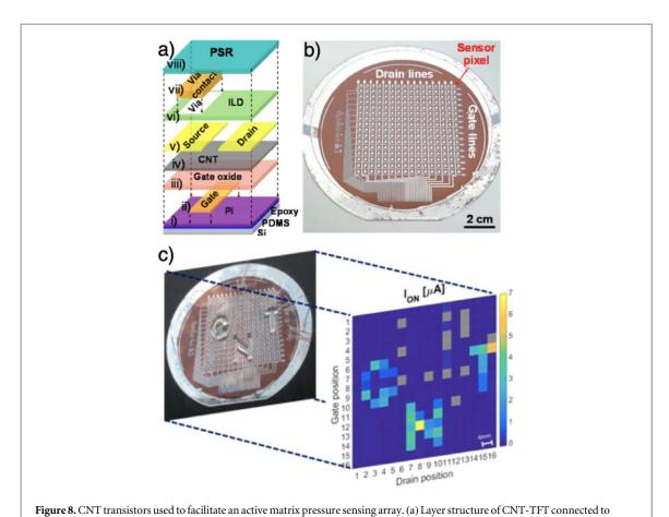
pressure-sensitive rubber. (b) Photograph of wafer-scale active matrix sensing array. (c) Demonstration of spatial mapping capability of the active matrix pressure sensor array. (a)–(c) are adapted from [28].
