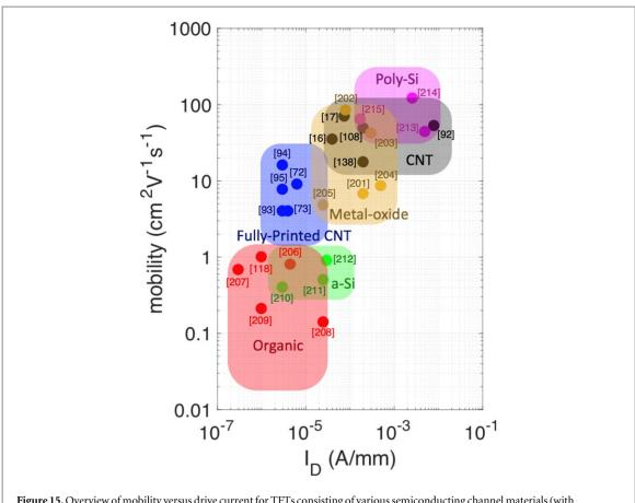
Figure 15. Overview of mobility versus drive current for TFTs consisting of various semiconducting channel materials (with  $V_{\rm DS} \leqslant 1$  V).
