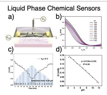
Figure 12. Poly(1-amino anthracene) functionalized CNT-TFT for pH sensing. (a) Schematic of the transistor device with solution-gating electrode. (b) Transfer curves of the device with respect to different pH in solution. (c) Transient response of the TFT at various pH under constant bias voltage. (d) Linear response of transconductance with respect to pH. (a)–(d) are adapted from [159].
