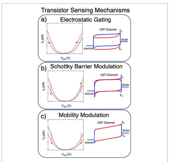
Figure 10. Sensing mechanisms of CNT-TFTs. Illustrated  $I_{\rm D}$ – $V_{\rm GS}$  curves for three of the most prominent CNT sensing schemes. (a) Electrostatic gating in which proximate charge modulates the potential of the CNT channel. (b) Schottky barrier modulation in which the metal-CNT barrier potential is modulated. (c) Mobility degradation due to creation of defects or trapped charge states within a CNT channel.
