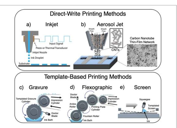
Figure 3. Methods for printing CNTs across both direct-write and template-based processes. (a) Schematic diagram and operation of an inkjet print head. (b) Schematic diagram of an aerosol jet printhead including device schematic with SEM image of CNT thin film. (b) Reproduced and adapted from [69]. Schematic diagrams of the (c) gravure, (d) flexographic, and (e) screen printing processes. (c)–(e) Reproduced and adapted from [70].
